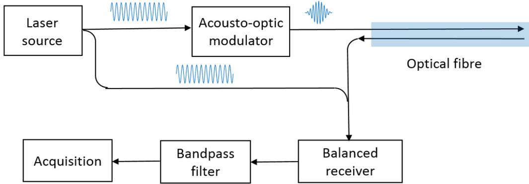
**Figure 1** Block diagram of the hDVS acquisition system.
