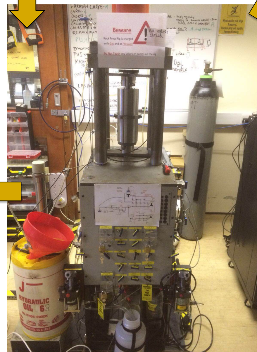
Image 1. Triaxial hydraulic deformation rig with oil flow control panel and chamber
