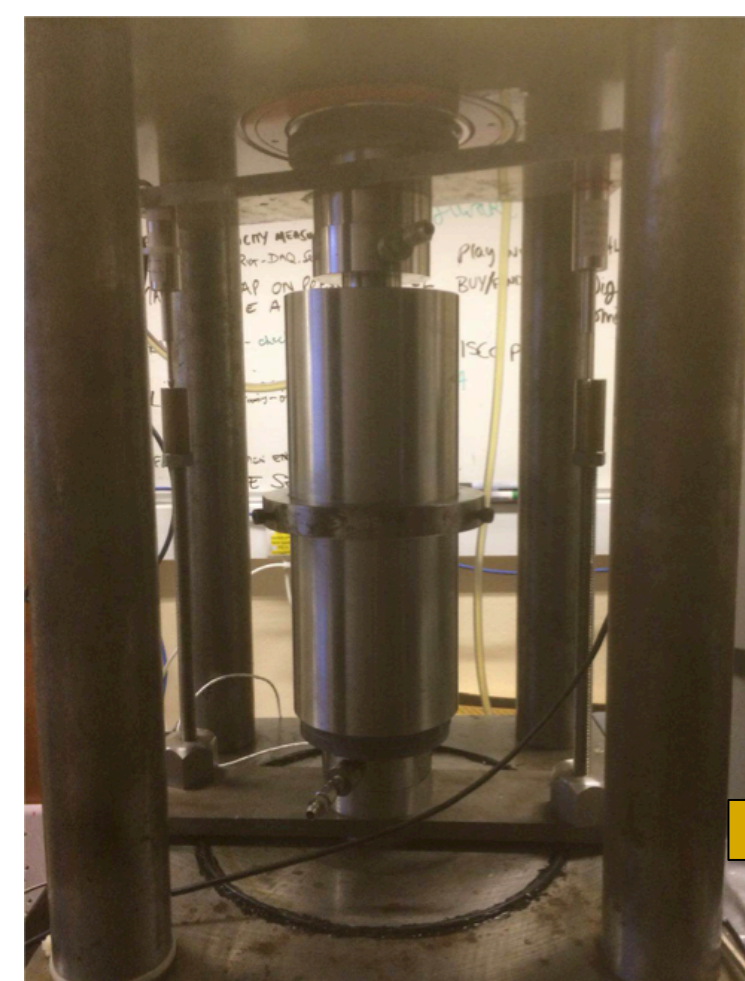
Image 2. Metal chamber mounted on rig with LVDT units running parallel
